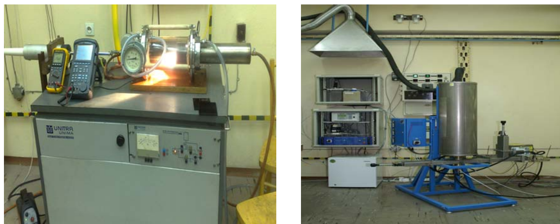
Fig.1 Arc plasma CNT synthesis – left and Microwave-CVD hybrid CNT synthesis - right
